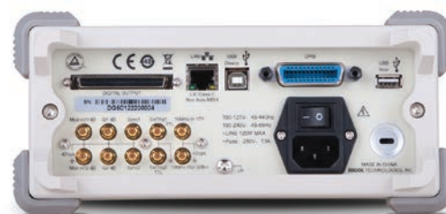
Complete connectivity, support Parallel Bus output (Option)
