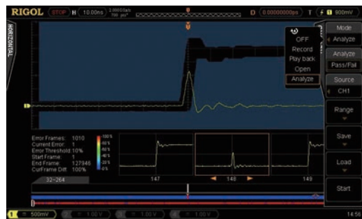
Real-time waveform record, replay, analysis function (Std.)
