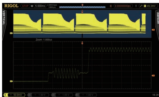
Deeper Memory with 256-Level intensity grading display
