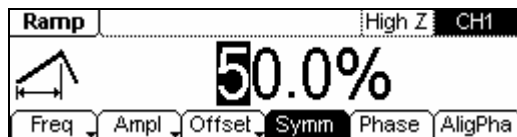
Figure 2-10 Ramp Signal Parameter Setting Interface
